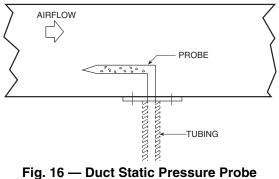
Fig. 16 — Duct Static Pressure Probe (P/N 39EK20462)
